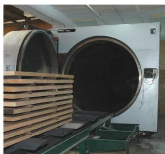
With the purpose to improve certain characteristics of the wood (coniferous as well as deciduous), it is submitted to heat treatment at high temperatures for a preset duration. The heat treatment is
